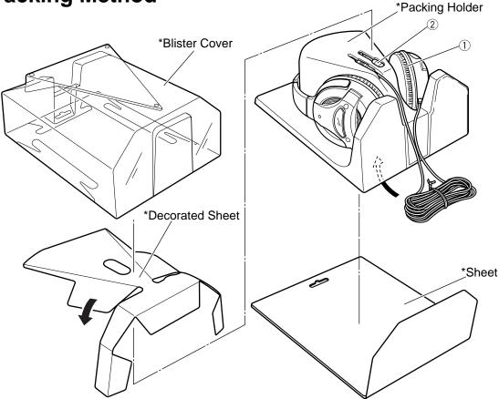
Note : These parts which was marked \*(Blister cover/ Decorated sheet/packing holder and sheet) will not be able to sypply as our service parts.
